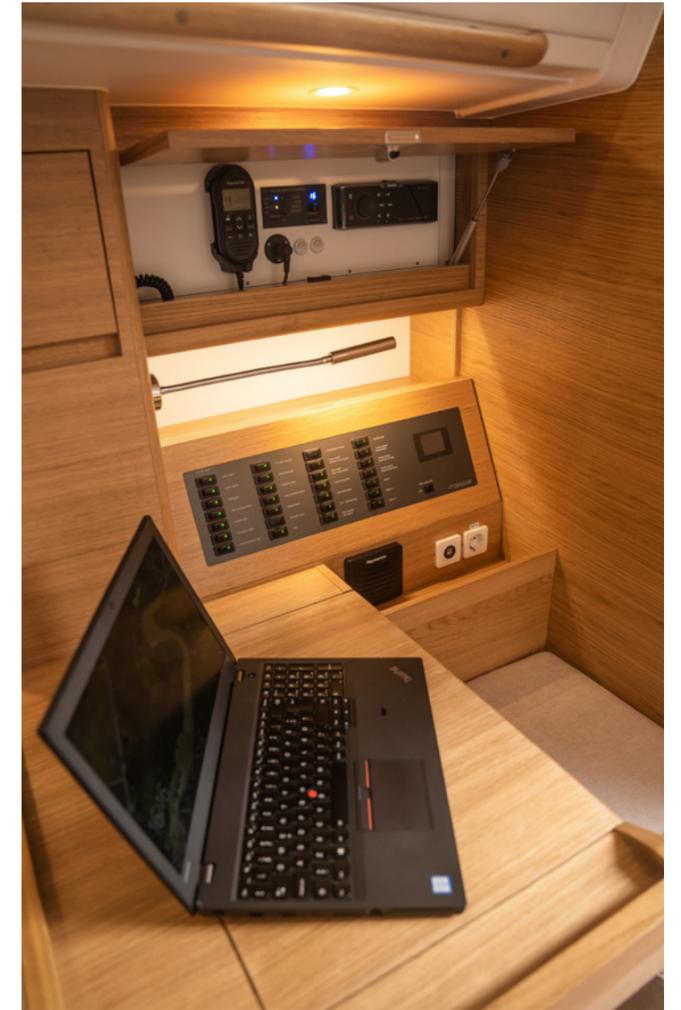
Above: The nav station is the X4<sup>6</sup>'s communication centre as well as the main hub for the yacht's electrical systems.
