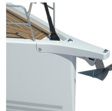
Optional carbon bowsprit, colour matched to hull with integrated anchor fitting.
